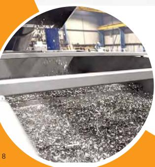
The screw leads onto the second vibrating sieve where the swarf will transfer across the screen to be dewatered and a final fines filter. This stage is crucial to reduce the moisture on the surface of the cut in preparation for the subsequent drying stage.
